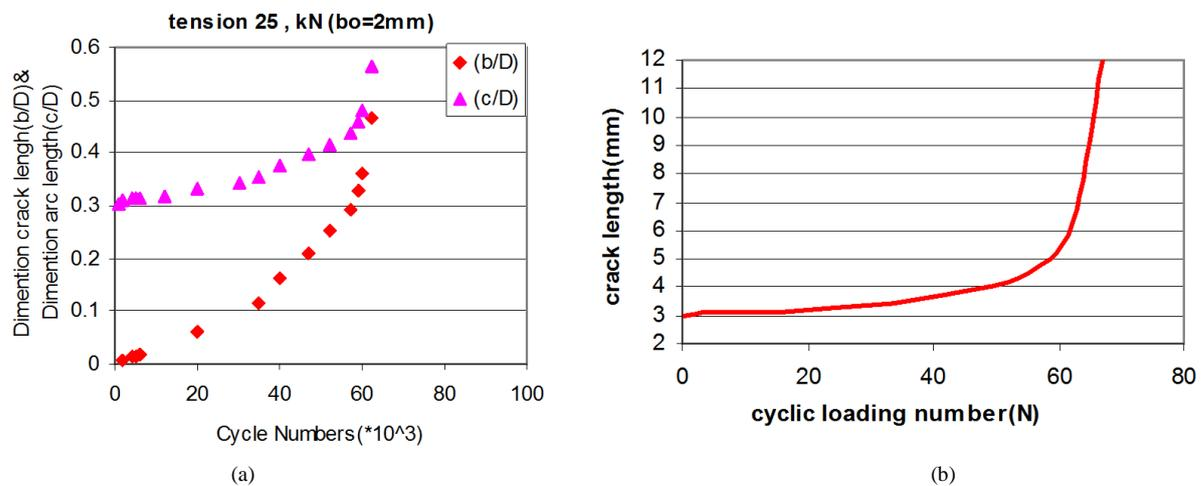
**Figure 5.** (a) Fatigue crack growth curves: arc length  $c$  versus cycle numbers  $N$ ; (b) Fatigue life curve of component.
