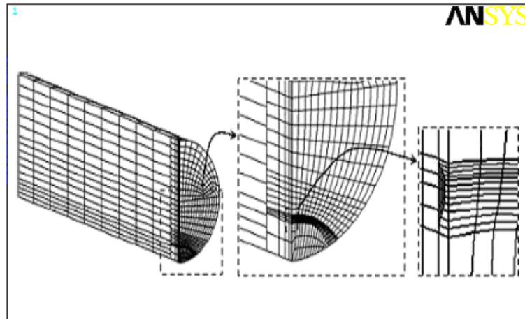
Figure 1. Three-dimensional model of cracked round bar.
