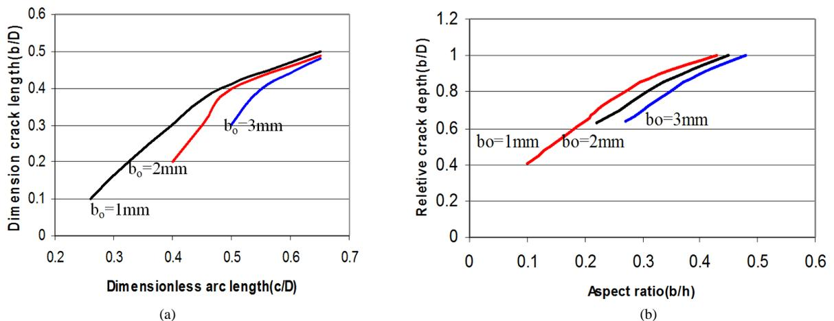
**Figure 4.** (a) Relationships of the crack growth in the depth and surface directions; (b) Fatigue crack growth patterns for different initial surface flaws.
