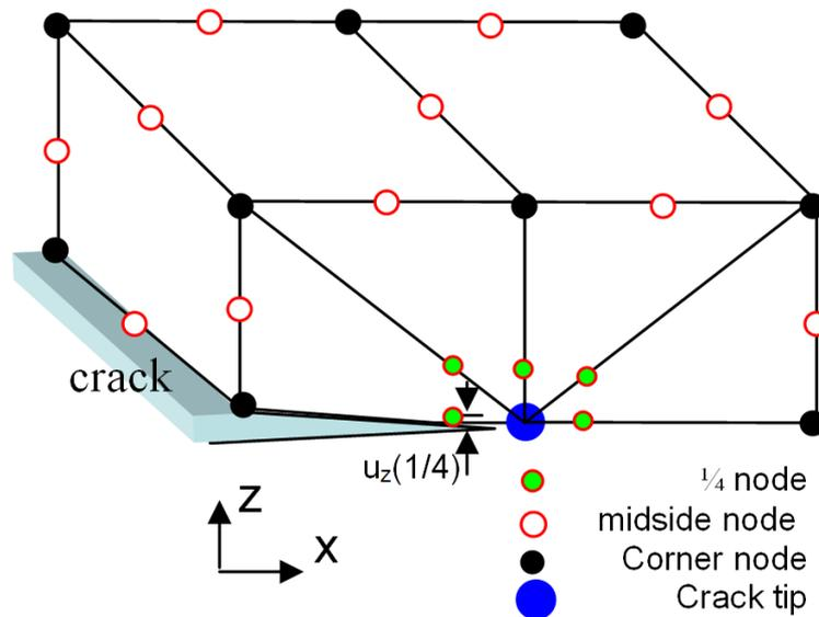
Figure 2. Mesh configuration near the crack tip.
