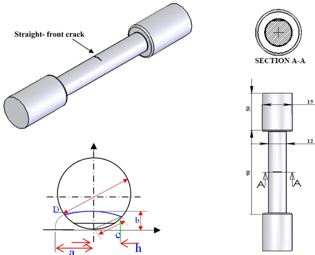
**Figure 3.** Details of the component geometry and crack.
