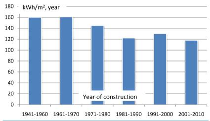
Figure 1. Energy use for heating and hot water in Swedish office buildings by year of construction (SEA, 2011).
