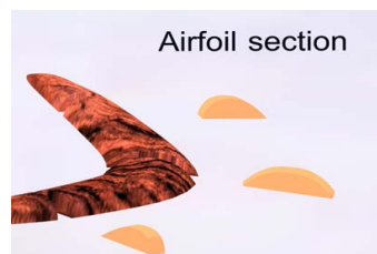
Figure 3. Different section views of the boomerang by which one can see how they vary depending on their relative position.
