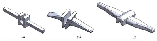
Figure 1. The geometries of the (a) Avanta (Sutter), (b) NeuFlex, (c) Swanson representative geometries, assembled in Solidworks and exported as solid meshes to ANSYS mechanical analysis. The dimensions used for developing the models were the same as those for the numerical analysis.
