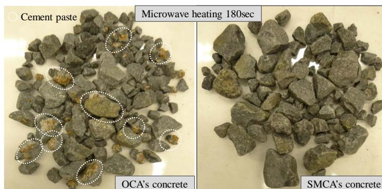
**Figure 19.** Comparison of RCA from each type of concrete.
