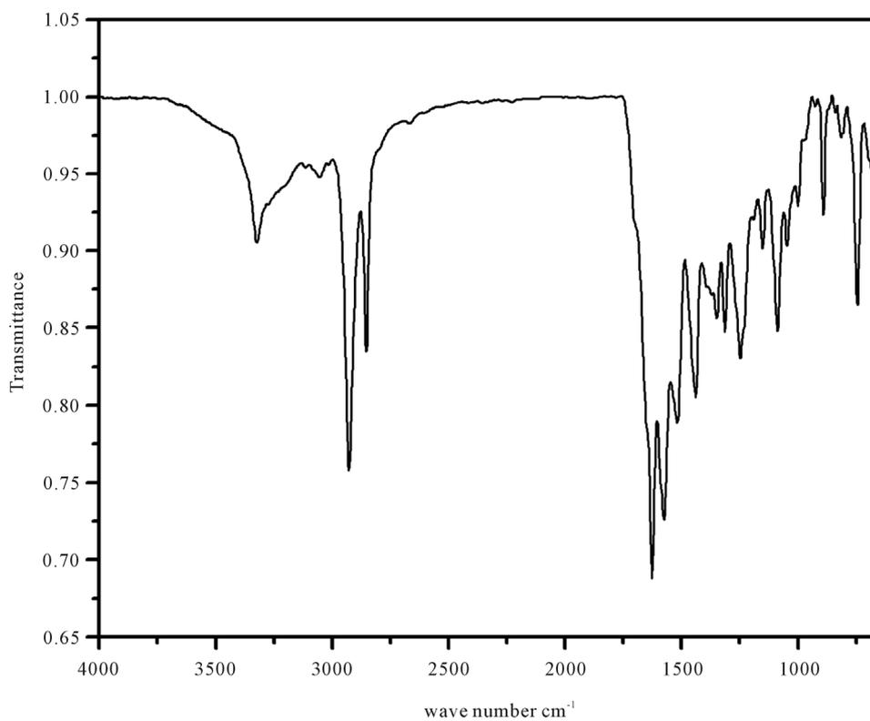
**Figure 9.** Infrared spectra of DPTR-II.
