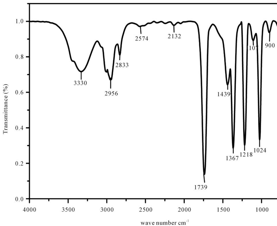
**Figure 10.** Infrared spectra of DPTY-II.
