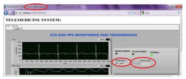
Figure 6. Web browser showing the front panel (RECEIVING SIDE).
