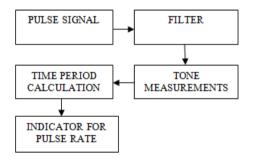
Figure 2. Block diagram for pulse rate detection.
