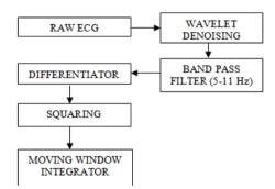
Figure 1. Block diagram for heart rate detection.
