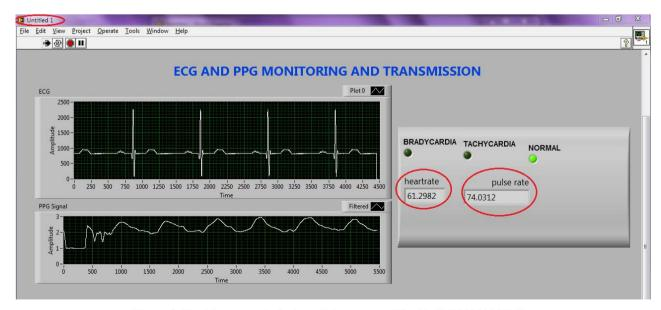
Figure 5. Final front panel of telemedicine system (TRAN- SMISSION SIDE).
