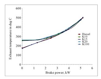
Figure 4. Variation of exhaust gas temperature with brake power.
