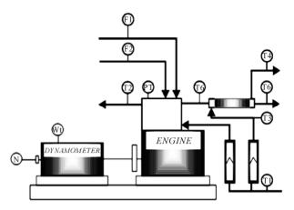
Figure 1. Engine test setup. PT-Pressure Transducer, N-Rotary encoder, Wt-Weight, F1-Fuel flow, F2-Air flow, F3-Jacket water flow, F4-Calorimeter water flow, T1-Jacket water inlet temperature, T2-Jacket water outlet temperature, T3-Calorimeter water inlet temperature, T5-Exhaust gas to calorimeter temperature, T6-Exhaust gas from calorimeter temperature.
