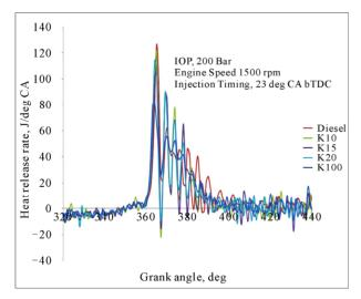
Figure 5. Variation of heat release rate with crank angle at full load.
