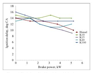
Figure 6. Variation of ignition delay with brake power.
