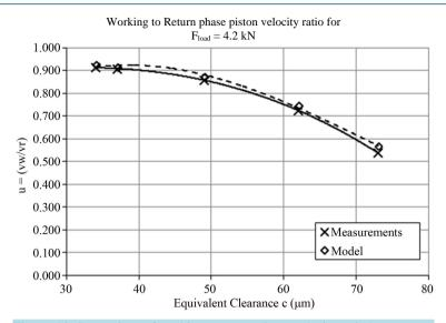
Figure 14. Comparison of working to return piston velocity ratio between experimental and model data for  $F_{load} = 4.2$  kN.
