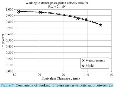
perimental and model data for  $F_{\text{load}} = 2.1$  kN.
