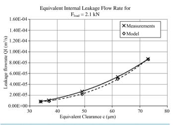
Figure 10. Comparison of equivalent leakage flow rate between experimental and model data for  $F_{\text{load}} = 2.1$  kN.
