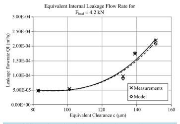
Figure 5. Comparison of equivalent leakage flow rate between experimental and model data for  $F_{\text{load}} = 4.2 \text{ kN}$ .
