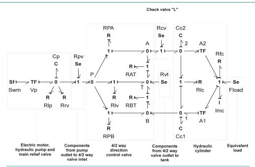
Figure 3. Hydraulic system bond graph model for the motion of the piston to the right.
