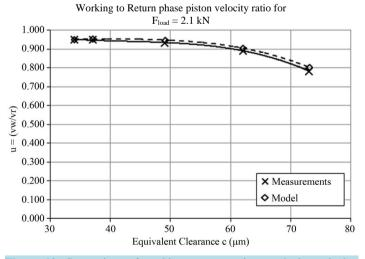
Figure 13. Comparison of working to return piston velocity ratio between experimental and model data for  $F_{\text{load}} = 2.1$  kN.
