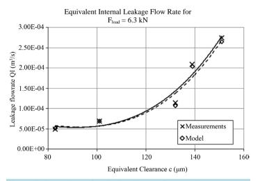
Figure 6. Comparison of equivalent leakage flow rate between experimental and model data for  $F_{\text{load}} = 6.3 \text{ kN}$ .
