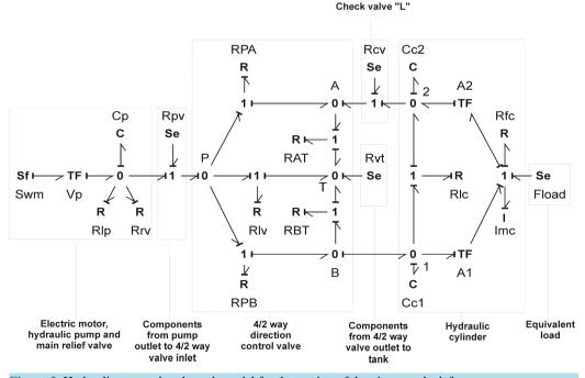
Figure 2. Hydraulic system bond graph model for the motion of the piston to the left.
