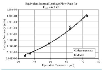
Figure 12. Comparison of equivalent leakage flow rate between experimental and model data for  $F_{\text{load}} = 6.3$  kN.
