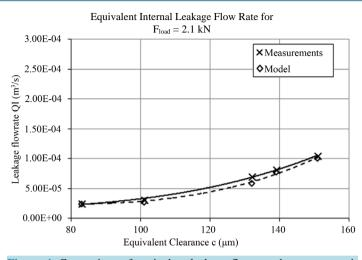
**Figure 4.** Comparison of equivalent leakage flow rate between experimental and model data for  $F_{\text{load}} = 2.1$  kN.
