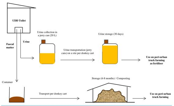
Figure 1. Flow of products (urine and feces) in the ecological sanitation system implemented in Ouagadougou.
