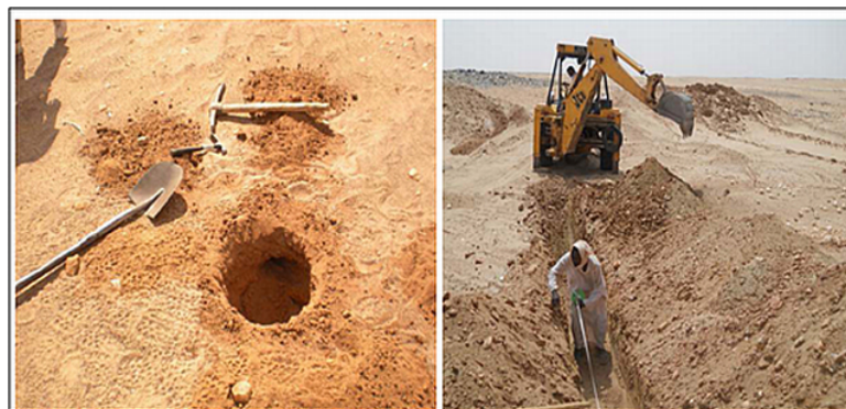
Figure 4. Process of pitting and trenching for sample collection in block I.
