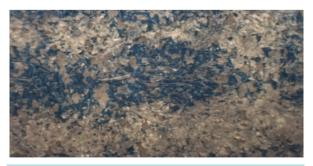
Figure 14. Photomacrograph of offset prints on paper coated with clay coating mixture containing MA/AA 10:90 binder At Magnification  $\approx 4 \times$ .
