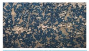
Figure 8. Photomacrograph of offset prints on paper coated with clay coating mixture containing MA/AA 90:10 binder. At Magnification  $\approx 4 \times$ .
