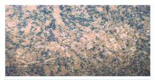
Figure 13. Photomacrograph of offset prints on paper coated with clay coating mixture containing MA/AA 30:70 binder. At Magnification  $\approx 4 \times$ .
