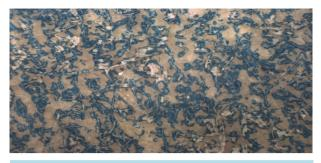
Figure 15. Photomacrograph of offset prints on paper coated with clay coating mixture containing MA/AA 1:2 binder. At Magnification  $\approx 4 \times$ .
