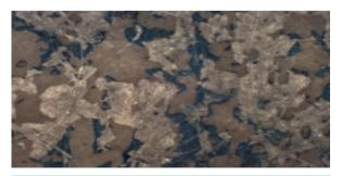
Figure 10. Photomacrograph of offset prints on paper coated with clay coating mixture containing MA/AA 70:30 binder At Magnification  $\approx 10 \times$ .
