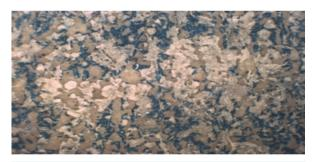
Figure 9. Photomacrograph of offset prints on paper coated with clay coating mixture containing MA/AA 70:30 binder. At Magnification  $\approx 4 \times$ .
