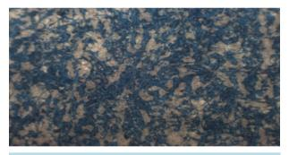
Figure 17. Photomacrograph of offset prints on paper coated with clay coating mixture containing (MA/AA + AMPS/AA) blend binder. At Magnification  $\approx 4 \times$ .
