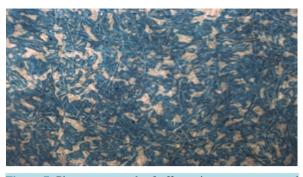
Figure 7. Photomacrograph of offset prints on paper coated with clay coating mixture containing commercial binder. At Magnification  $\approx 4 \times$ .
