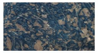
Figure 12. Photomacrograph of offset prints on paper coated with clay coating mixture containing MA/AA 50:50 binder. At Magnification  $\approx 10 \times$ .
