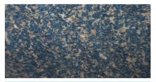
Figure 11. Photomacrograph of offset prints on paper coated with clay coating mixture containing MA/AA 50:50 binder. At Magnification  $\approx 4 \times$ .
