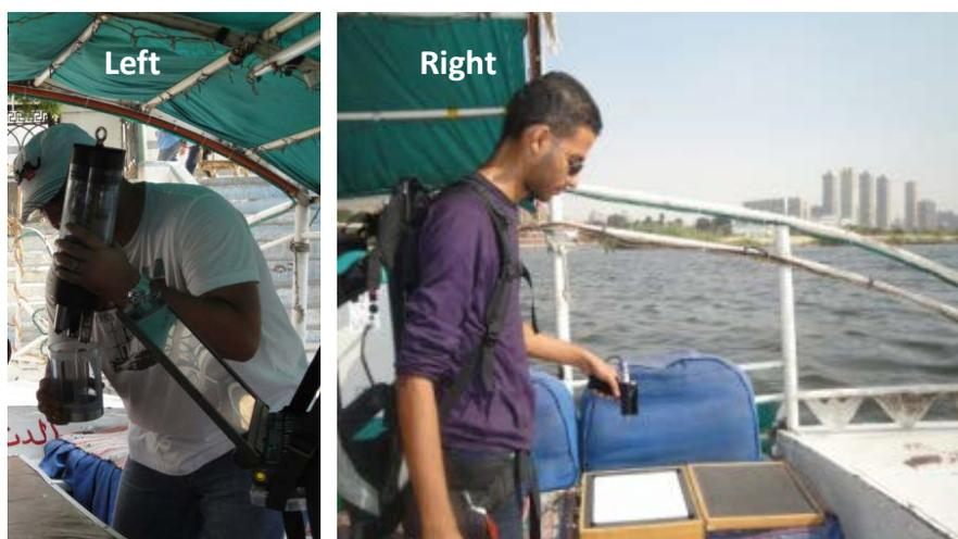
**Figure 2.** Field picture of the *in-situ* measurement devices (right = ASD spectroradiometer, left = eco-sounder multi-probe).
