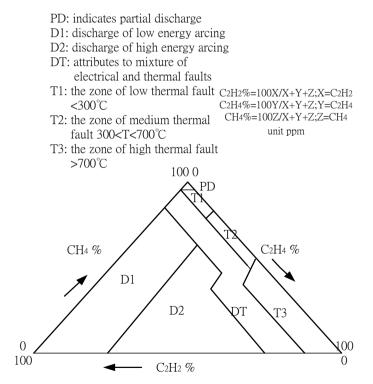
Figure 2. IEC-Duval triangle method [3].
