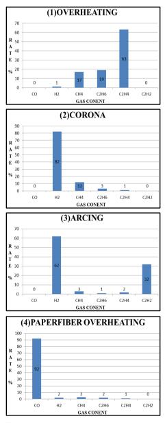
**Figure 1.** The gas content of typical faults proportion.
