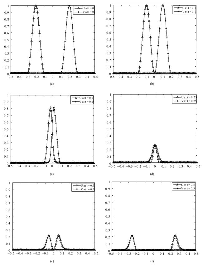
Figure 3. Numerical solution using quintics. Figures 3(a)-3(f) show the motion and interaction of the waves u and v.
