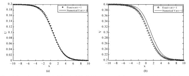
Figure 2. Comparison of numerical solution using RK4 with MQ versus exact solutions *u*, *v* at time t = 1 when  $\alpha = 1$ ,  $\beta = 2$ ,  $a_0 = 0.1$ , c = 0.58 and  $\delta_t = 0.001$ , corresponding to Problem 2.
