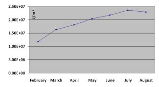
Figure 2. Monthly average daily radiation using data from 9 station in Iran.
