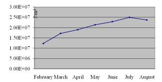
Figure 1. Estimate monthly average daily solar radiation using Montis cofficients.
