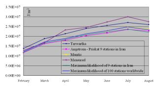
Figure 7. Compares model types of Angstrom-Pryskat and Maximum likelihood.
