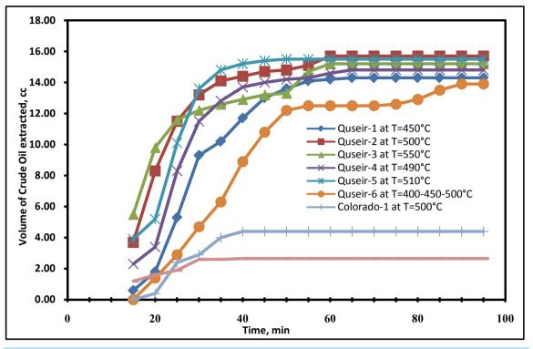
Figure 6. Relationship between volumes of Oil extracted versus Time for different shale oil samples.
