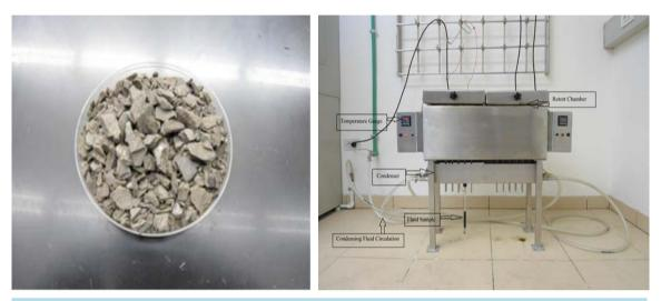
Figure 4. Crushed sample for oil shale and put in the retort at different temperatures.
