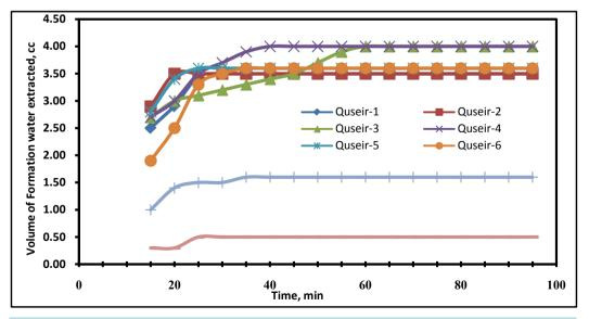
Figure 5. Relationship between volumes of formation water extracted versus time for different shale oil samples.
