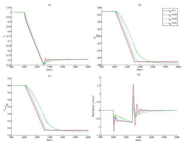
Figure 3. Numerical simulation results: (a) Relative nuclear power, (b) Average fuel temperature, (c) Outlet helium temperature, (d) Designed control rod speed signal.
