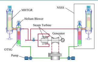
Figure 1. Composition of the HTR-PM plant.
