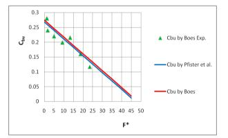
Figure 3. Comparison of uniform bottom air concentration  $(C_{bu})$ .
