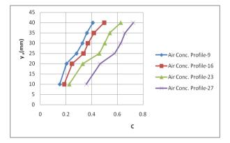
Figure 1. Air concentration profiles on stepped spillway model ( $q = 0.0400 \text{ m}^3/\text{s}\cdot\text{m}$ ).
