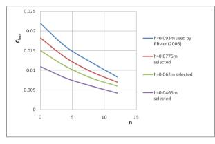
Figure 5. Variation of  $C_{bm}$  with step number for  $q = 0.866 \text{ m}^3/\text{s}\cdot\text{m}$ .
