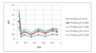
Figure 6. Mean pressure profiles on stepped spillway model.
