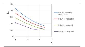
Figure 4. Variation of  $C_{bm}$  with step number for  $q=0.109\ m^3/s{\cdot}m.$
