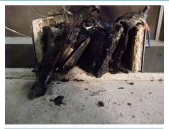
Figure 11. Module of 4 cells after overcharge of a single cell.
