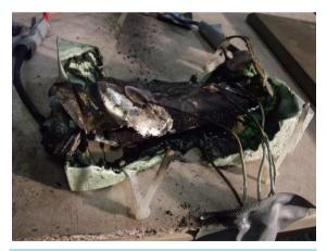
Figure 6. Destroyed overcharge cell after the test, burned and ruptured.
