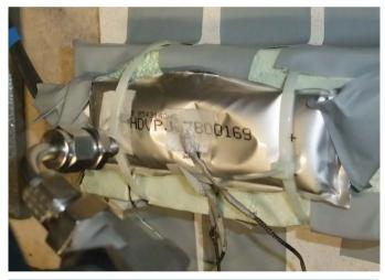
Figure 8. Cell after emergency cooling experiment. Cell inflated and the  $CO_2$  pulse resulted in a dented cell. No cell rupture occurred.
