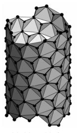
Figure 11. The polyhedric model of a nanotube with the diameter D = 8.47 Å, the chirality angle  $\beta = 46.1^{\circ}$  and the roll up direction v = [4,3].
