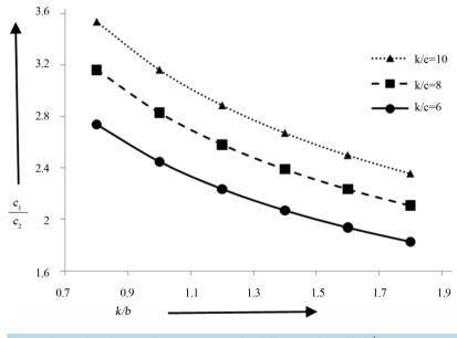
**Figure 2.** Torsional wave dispersion curve for different values of k/c.
