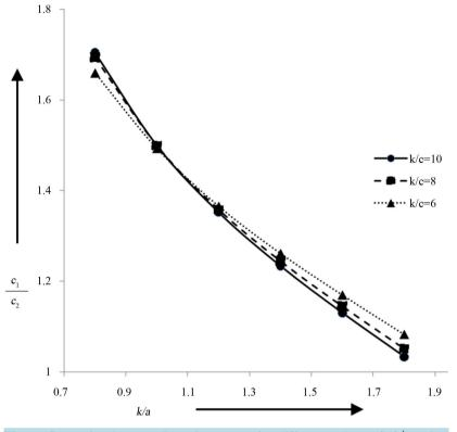
**Figure 5.** Torsional wave dispersion curve for different values of k/c when k/b = 2.
