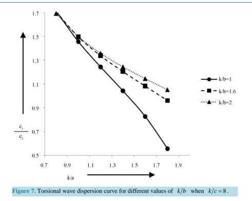
of the medium increases, the velocity of the torsional wave decreases. In the lower ranges of rigidity, the dispersions of torsional surface waves are less significant as compared to the higher ranges. Also from **Figure 7**, it has been shown that the longitudinal and transverse rigidity has inverse effect in the propagation of torsional surface waves in the medium of fixed density. Lastly when the medium is homogeneous and isotropic in nature, torsional surface wave does not propagate there.
