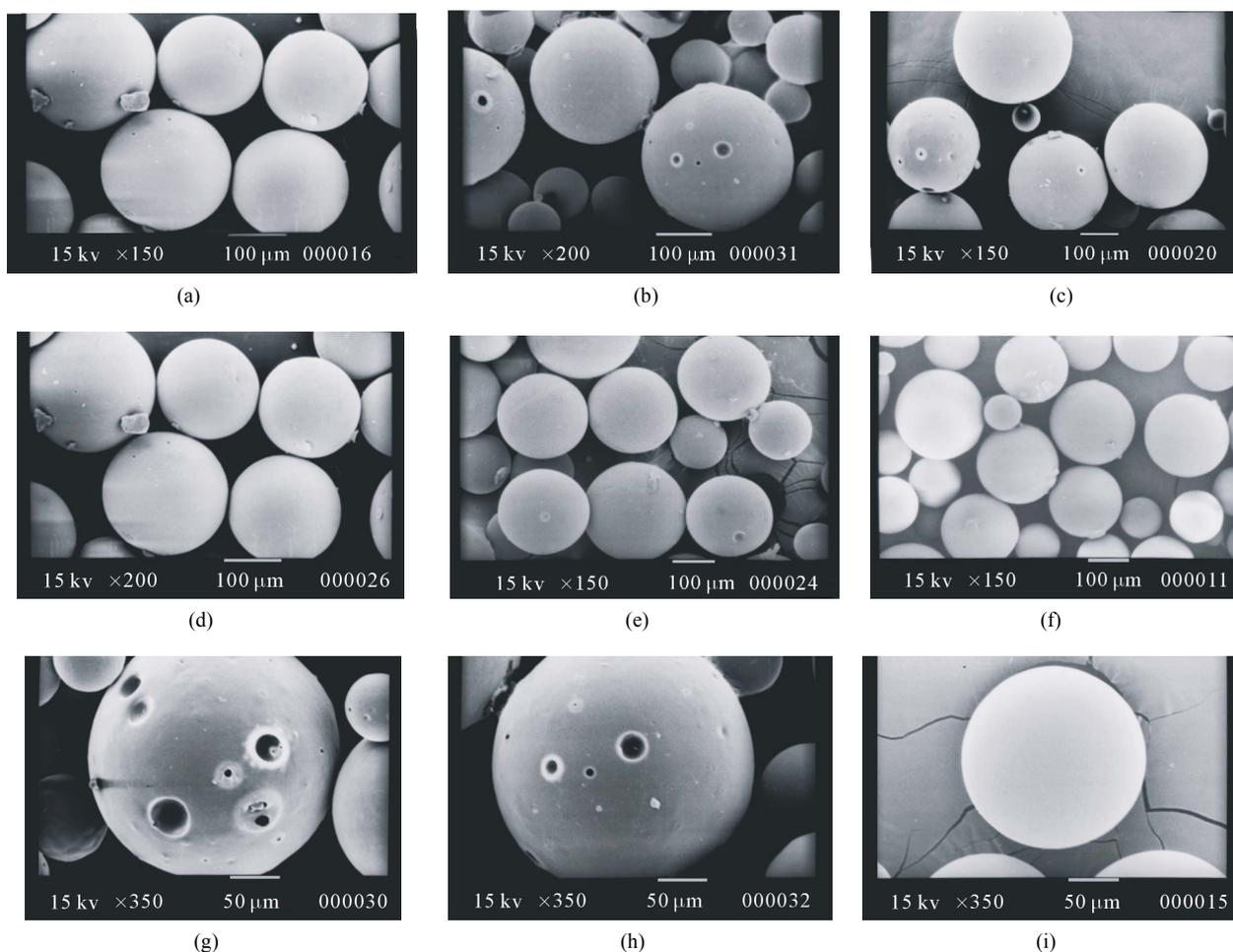
**Figure 3.** Scanning electron micrographs of: non-matrix microcapsules prepared with different volume of  $W_1$  phase (3 ml - a, 5 ml - b, 7 ml - c); matrix microcapsules prepared with 4% w/v PMMA and different concentration of SAL (0.5% - d, 1.5% - e, 2.5% - f); matrix microcapsules prepared with 2% w/v SAL in  $W_1$  phase and different concentration of PMMA (2% - g, 3% - h, 4% - i).
