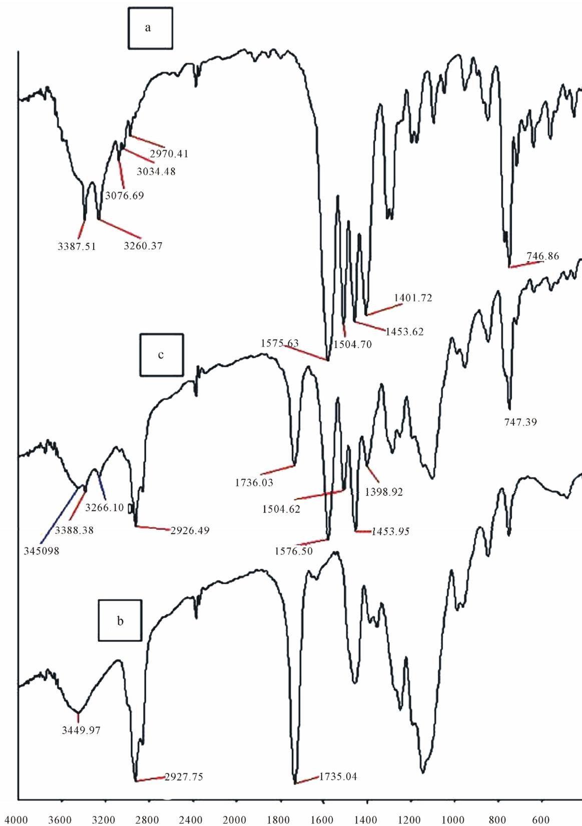
Figure 1. FTIR spectra of (a) diclofenac sodium, (b) blank microcapsules, (c) drug loaded microcapsules.
