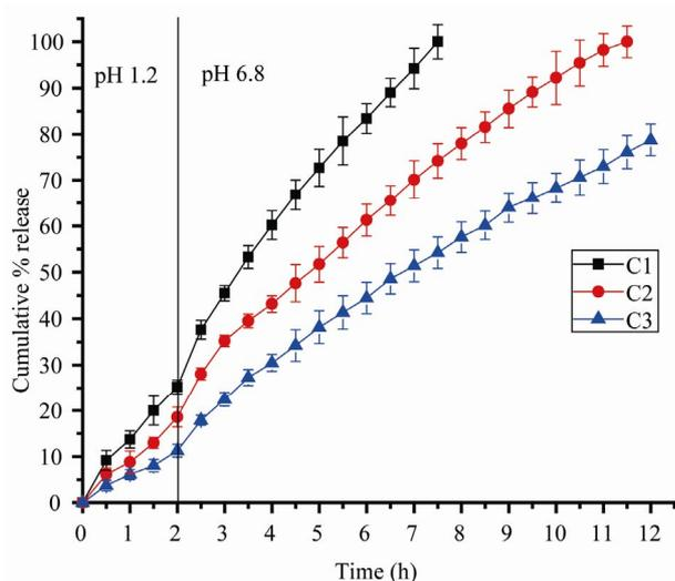
**Figure 4.** Release profiles of diclofenac sodium from matrix microcapsules prepared with 2% w/v SAL in  $W_1$  phase and different concentration of PMMA (2% - C1, 3% - C2, 4% - C3).
