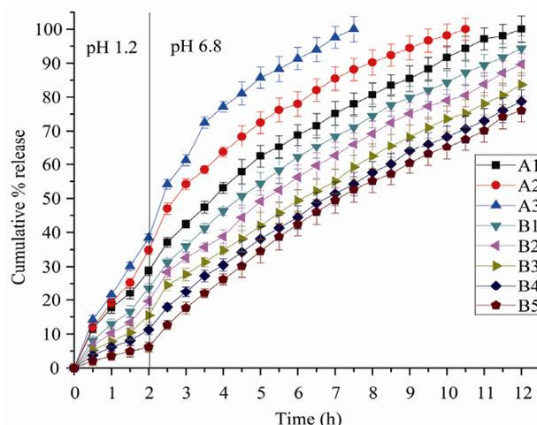
Figure 2. Release profile of diclofenac sodium from non-matrix microcapsules prepared with different volume of  $W_1$  phase (3 ml - A1, 5ml - A2, 7ml - A3) and matrix microcapsules prepared with different concentration of SAL in  $W_1$  phase (0.5% - B1, 1.0% - B2, 1.5% - B3, 2.0% - B4, 2.5% - B5).
