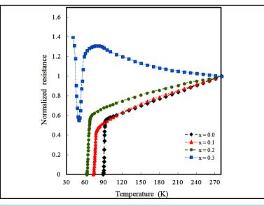
**Figure 3.** Variation of normalized resistance with temperature of  $Y_1Ba_2Cu_{3-x}Pr_xO_{7-\delta}$  samples with x = 0.0, 0.1, 0.2, and 0.3.
