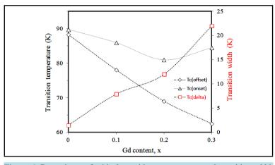
**Figure 6.** Dependence of critical transition temperatures and transition width on Gd-content, *x*, of prepared  $Y_1Ba_2Cu_{3-x}Gd_xO_{7-\delta}$  samples.
