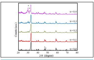
**Figure 2.** Normalized XRD pattern of  $Y_1Ba_2Cu_{3-x}Gd_xO_{7-\delta}$  samples with x = 0.0, 0.1, 0.2, 0.3, and 0.4. The peaks denoted by (+) referred to  $Y_2BaCuO_5$  phase while (\*) peaks referred to (020) and (200) indices.
