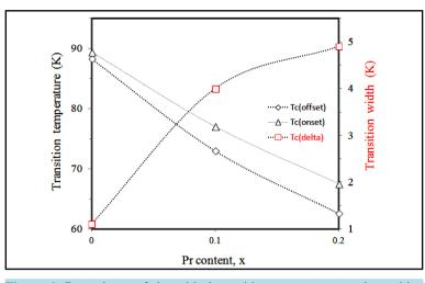
**Figure 4.** Dependence of the critical transition temperatures and transition width on Pr-content, *x*.
