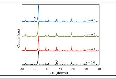
**Figure 1.** Normalized XRD pattern of  $Y_1Ba_2Cu_{3-x}Pr_xO_{7-\delta}$  with x = 0.0, 0.1, 0.2, and 0.3. The peaks denoted by (+) referred to  $Y_2BaCuO_5$  phase while (\*) peaks referred to (020) and (200) indices.
