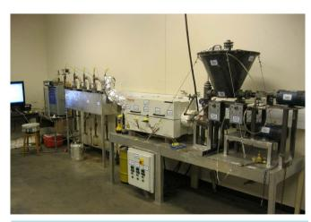
Figure 1. The allothermal auger gasification system.
