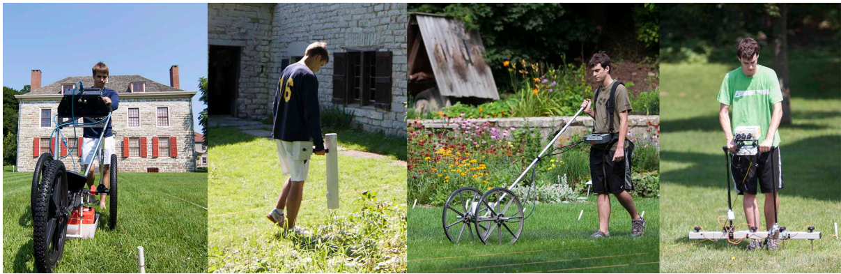
Figure 5. Archaeogeophysical instruments used at Old Fort Johnson and Fort Klock; from Left to Right: GSSI SIR 3000 GPR with 400 MHz antenna, Geoscan FM256 Fluxgate gradiometer, Geometrics G-858 dual cesium gradiometer, Geoscan RM15 earth resistance meter with multiplexer.
