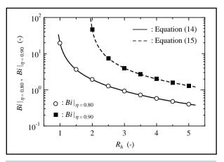
Figure 8. Biot number index to use 45° heat spreading angle.
