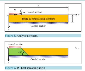
where  $\lambda$  is the thermal conductivity of the board, *q* the heat flux from the heat source,  $\alpha$  the heat transfer coefficient at the cooled section and *T*<sub>f</sub> the cooling fluid temperature. The following adiabatic boundary condition is applied at the surfaces except for the heated and the cooled section:
