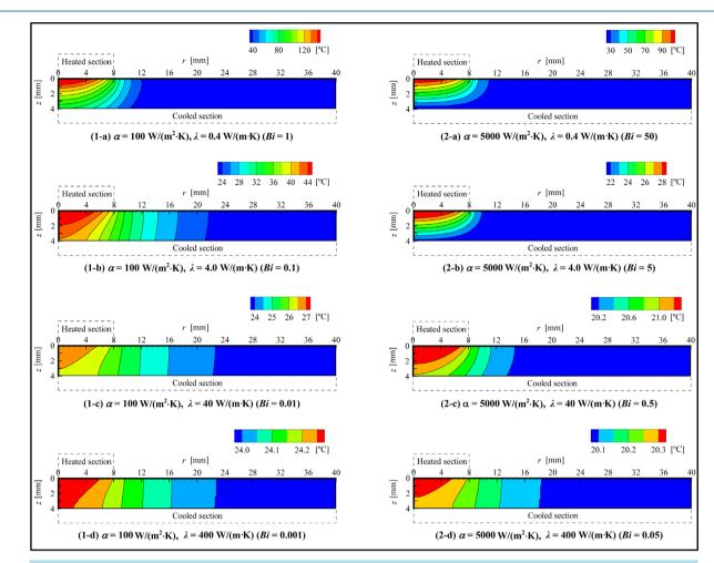
**Figure 3.** Temperature distribution inside board ( $r_h = 8 \text{ mm}$ ,  $r_c = 40 \text{ mm}$ ).
