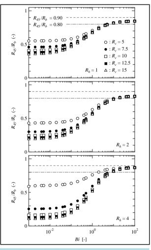
**Figure 9.** Thermal resistance of board: comparison between 45° heat spreading approach and numerical results.
