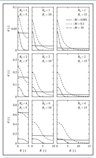
Figure 5. Dimensionless temperature distribution at cooled section.
