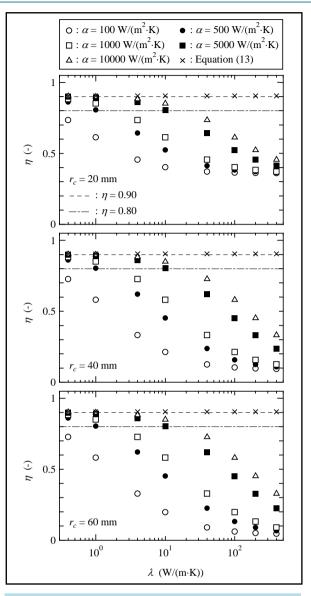
**Figure 6.** 45° heat spreading characteristics ( $r_h = 8$  mm).
