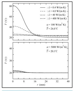
**Figure 4.** Temperature distribution at cooled section ( $r_h = 8 \text{ mm}, r_c = 40 \text{ mm}$ ).
