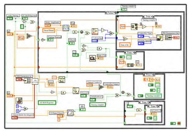
Figure 6. PID auto-tuning (all features) block diagram.
