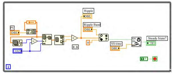
Figure 8. SS test block diagram.
