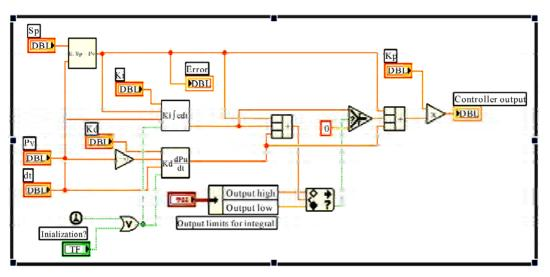
Figure 13. PID controller block diagram.
