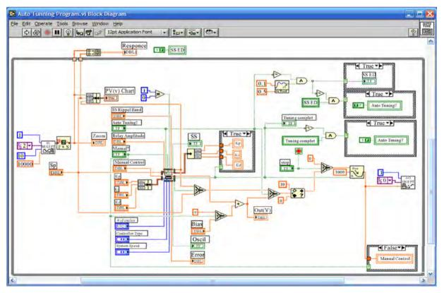
Figure 4. PID auto-tuning VI block diagram.
