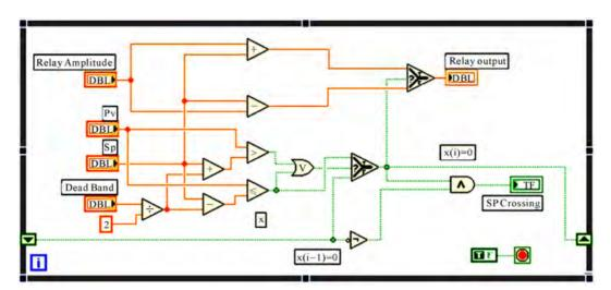
Figure 12. SP relay block diagram.
