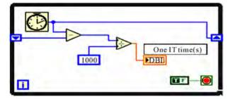
Figure 11. Find iteration time (dt) block diagram.
