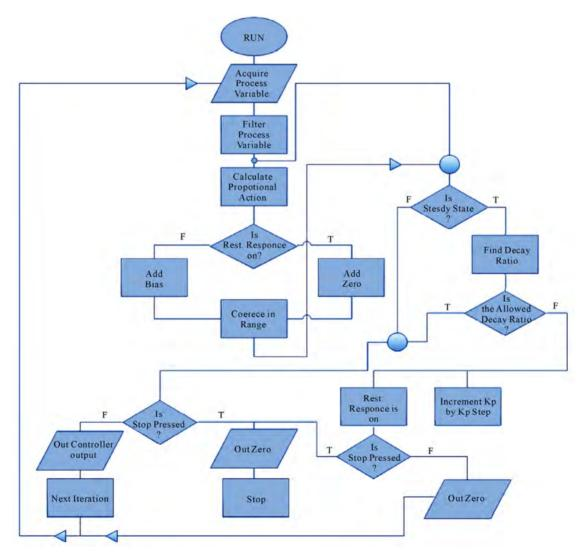
Figure 2. PID auto-tuning VI flow chart.
