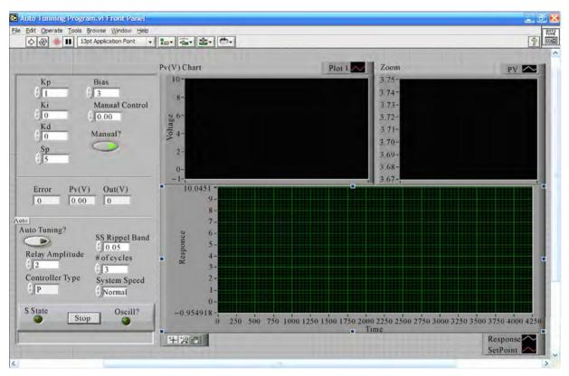
Figure 3. The front panel of PID auto-tuning VI.
