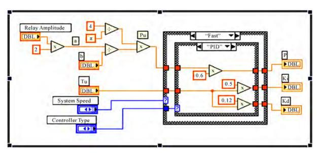
Figure 9. Calculate best PID parameters block diagram.
