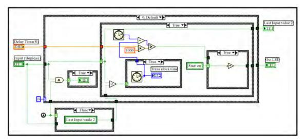
Figure 1. On-delay timer block diagram.
