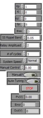
The PID auto-tuning (all features) SubVI is shown in **Figure 6**. It includes the following SubVIs:
