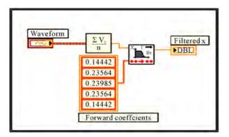
Figure 15. Filtering & smoothing waveform block diagram.
