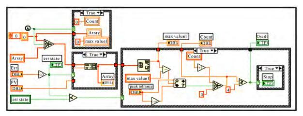
Figure 10. Check oscillation block diagram.
