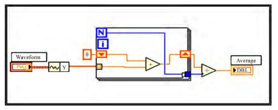
Figure 16. Waveform values average block diagram.
