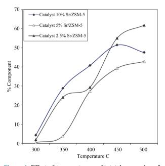
Figure 4. Effect of temperature on % total conversion of alkylation of toluene on different catalysts.
