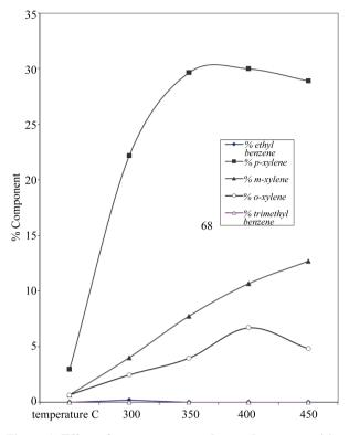
Figure 1. Effect of temperature on the product composition on 10% Sr/ZSM-5.
