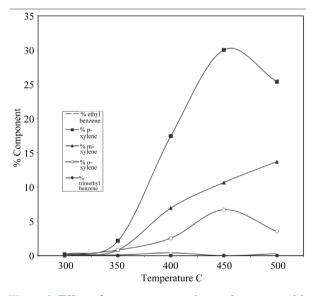
**Figure 2.** Effect of temperature on the product composition on 5% Sr/ZSM-5.
