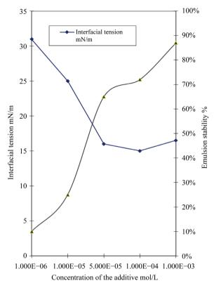
Figure 5. Effect of concentration of the additive on interfacial tension of toluene/methanol and emulsion stability.
