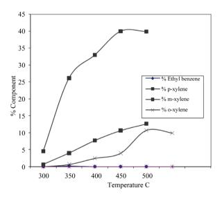
**Figure 6.** Effect of temperature on the product composition on the modified 10% Sr/ZSM-5.
