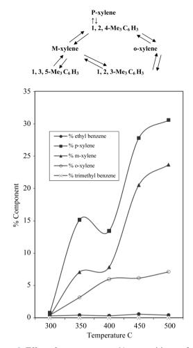
Figure 3. Effect of temperature on % composition on 2.5% Sr/ZSM-5.
