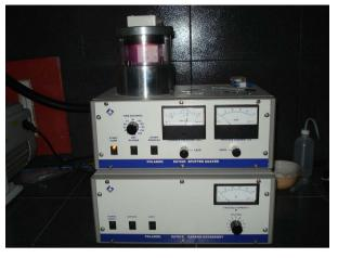
Figure 3. Evaporating metal coating (Au-Pd) in non-conductive samples.
