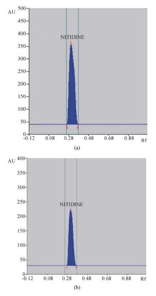
Figure 2. Typical HPTLC densitogram of nitidine in standard (a) and sample (b).
