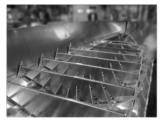
Figure 2. Hull of an aluminum boat and its internal stiffener structure.
