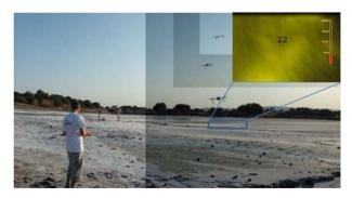
Figure 6. The frame composite visible image shows the reconstructed pattern of the second hexacopter flight. Inset shows the frame from the drone-borne thermal camera taken on the same site as field temperature measurements and the temperature measured in the centre of the image.
