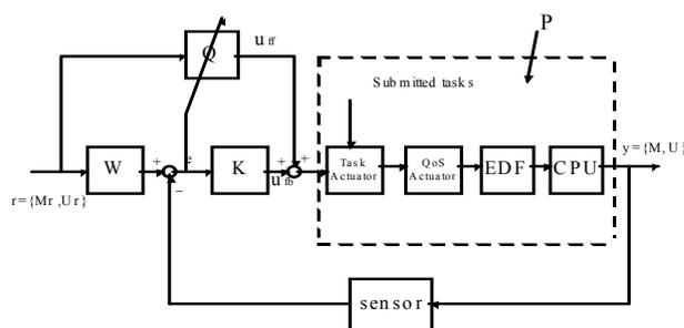
Figure 1. Architecture of FEL-H control scheduling
