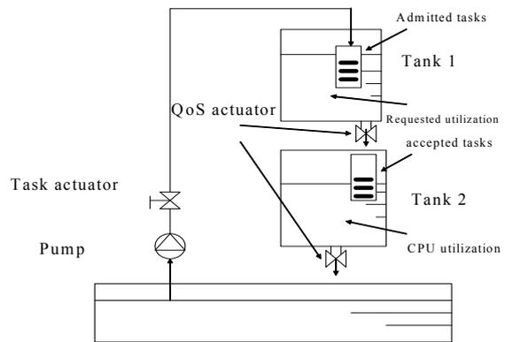
Figure 2. Two-tank system model of a scheduling system
