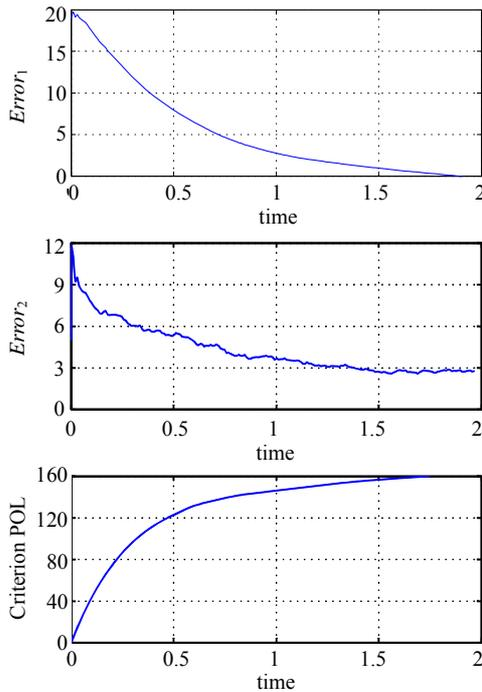
**Figure 2.** Graphs of the  $Error_1$ ,  $Error_2$ , and exponential mean square cost criterion corresponding to the polynomial filtering equations for a continuous stirred tank reactor for  $\varepsilon = 10$ ,  $X_1(0) = 20$ ,  $X_2(0) = 10$ ,  $Y_1(0) = 2$ ,  $Y_2(0) = 1$ .
