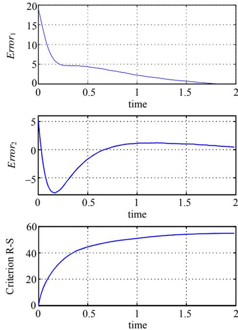
**Figure 1.** Graphs of the  $Error_1$ ,  $Error_2$ , and exponential mean square cost criterion corresponding to the risk-sensitive optimal filtering equations for a continuous stirred tank reactor for  $\varepsilon = 10$ ,  $X_1(0) = 20$ ,  $X_2(0) = 10$ ,  $Y_1(0) = 2$ ,  $Y_2(0) = 1$ .
