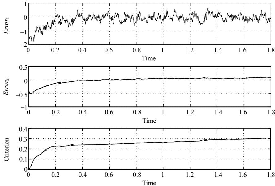
Figure 5. Graphs of the  $Error_1$ ,  $Error_2$ , and exponential mean square cost criterion corresponding to the polynomial filtering equations for satellite monoaxial for  $\varepsilon = 10$ ,  $X_1(0) = 0.115$ ,  $X_2(0) = 0.073$ ,  $Y_1(0) = 2$ ,  $Y_2(0) = 1$ .
