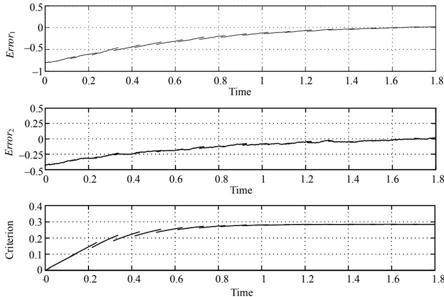
**Figure 4.** Graphs of the  $Error_1, Error_2,$  and exponential mean square cost criterion corresponding to the risk-sensitive optimal filtering equations for satellite monoaxial for  $\varepsilon = 10, X_1(0) = 0.115, X_2(0) = 0.073, Y_1(0) = 2, Y_2(0) = 1.$
