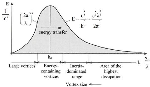
Figure 2. Energy spectrum as function of the wave number.
