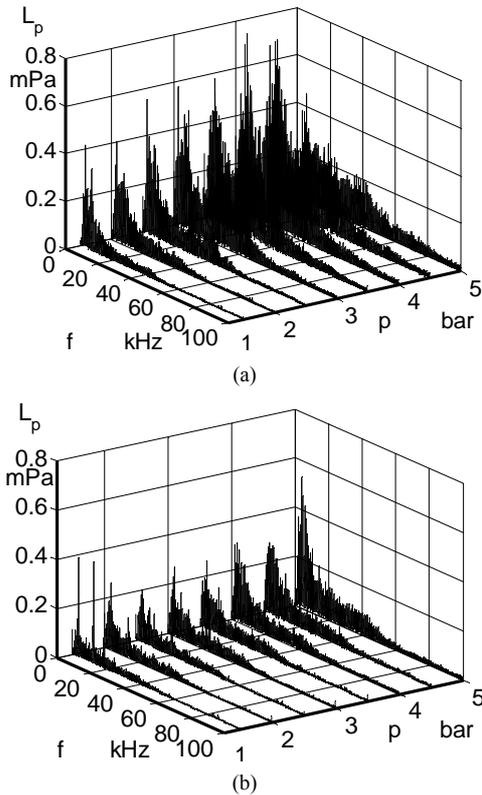
**Figure 5.** Fast Fourier transforms (FFT) of the sound pressure for the pressures from  $p = 1.0$  bar up to  $5.0$  bar at  $d = 10$  mm and  $d = 18.4$  mm.
