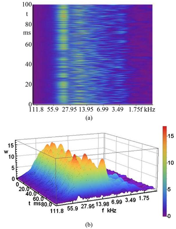
Figure 12. Plane and three-dimensional Gabor wavelet for the sound pressure at  $d = 3$  mm and  $p = 4.25$  bar.
