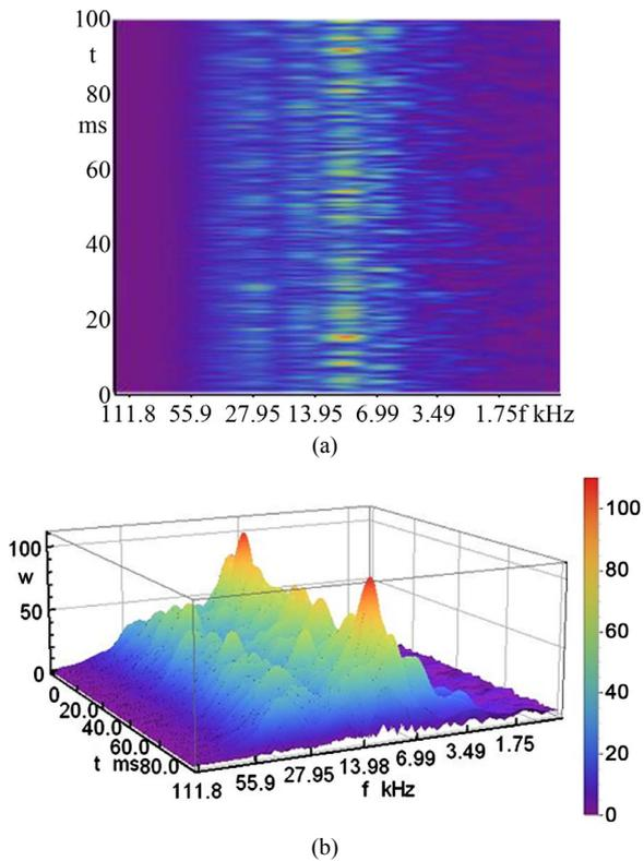
Figure 11. Plane and three-dimensional Gabor wavelet for the sound pressure at  $d = 2.0$  mm and  $p = 5$  bar.
