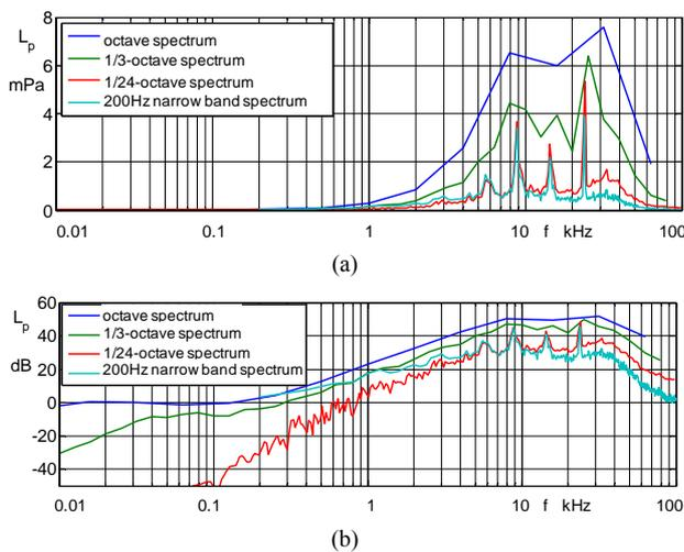
**Figure 6.** Spectra of the sound pressure (a) and of the pressure level (b) for the octave spectrum till the narrow band spectrum for  $d = 2$  mm,  $L = 12$  mm and  $p = 5$  bar.
