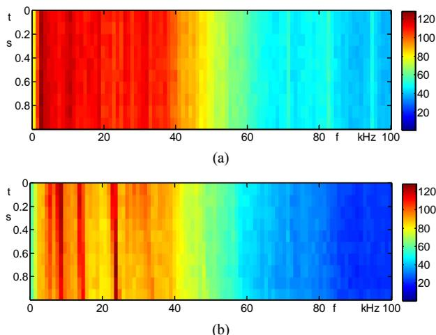
**Figure 8.** (a) Spectrogram for the diameter  $d = 1$  mm,  $L = 12$  mm and pressure  $p = 3$  bar; (b) Spectrogram for the diameter  $d = 2$  mm,  $L = 12$  mm and pressure  $p = 5$  bar.
