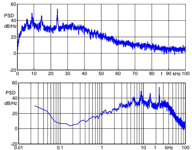
**Figure 9.** Power spectral density in linear and logarithmic scale for  $d = 2$  mm,  $L = 12$  mm and  $p = 5$  bar.
