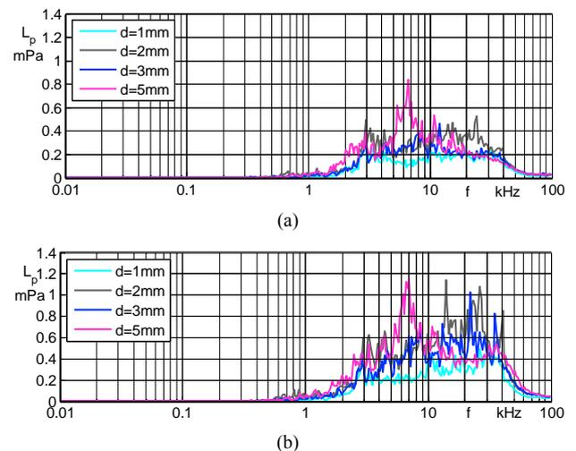
**Figure 7.** Comparing the 1/24 octave spectra of the sound pressure for openings of  $d = 1$  mm up to  $5$  mm and pressures of  $p = 2.0$  bar (a) and  $3.0$  bar (b).
