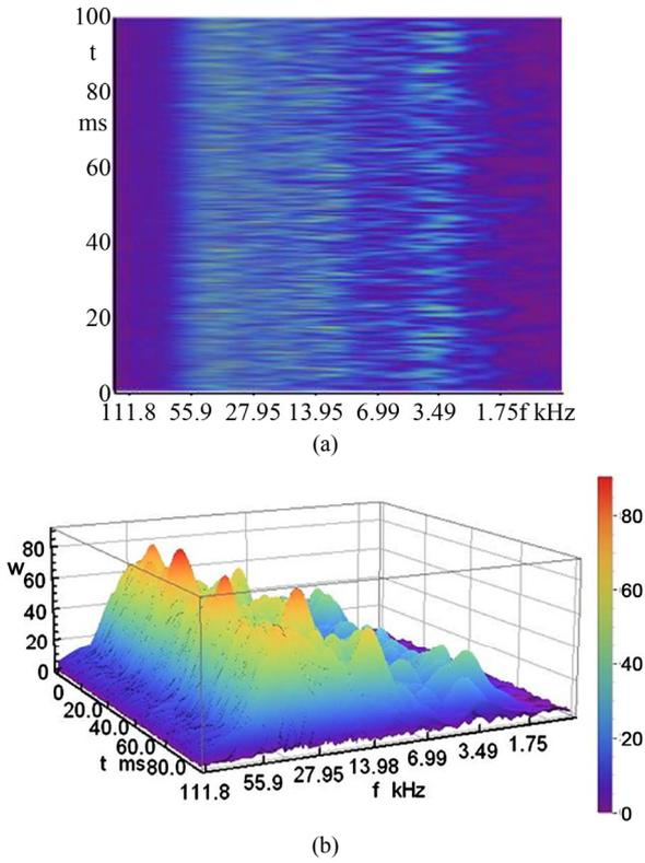
Figure 10. Plane and three-dimensional Gabor wavelet for the sound pressure at  $d = 1.6$  mm and  $p = 5$  bar.
