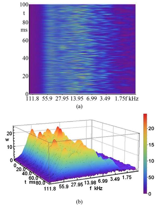
Figure 13. Plane and three-dimensional Gabor wavelet for the sound pressure at  $d = 4$  mm and  $p = 5$  bar.
