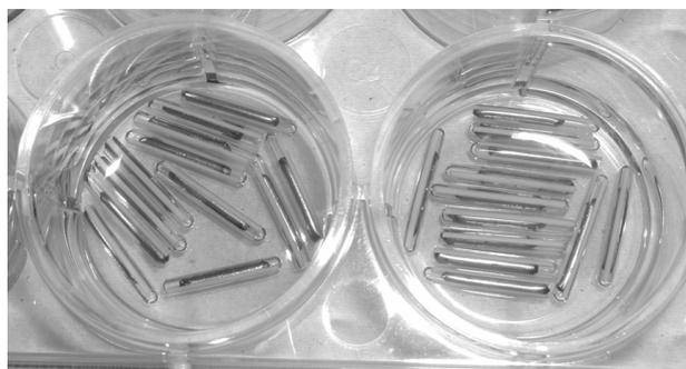
**Figure 1.** Catheter and stainless steel pieces forming load on HUVEC in a 12-well plate.
