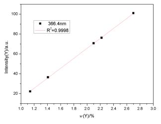
Figure 4. Calibration curve for Y II 366.4 nm.
