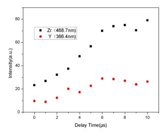
Figure 2. Intensity vs. gate delay time for the Y II 366.4nm and Zr I 468.7nm (#56).
