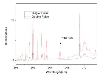
Figure 3. Comparison of DP-LIBS signalintensity with single pulse LIBS for Y (#56).
