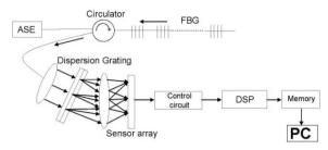
Figure 1. Schematic diagram of temperature demodulation system.
