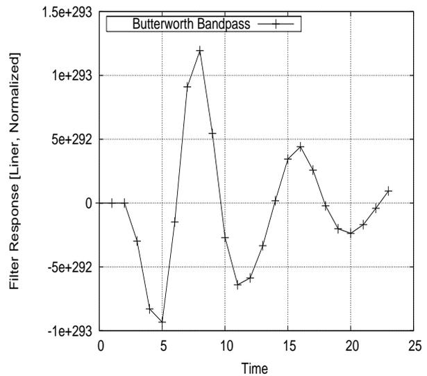
**Figure 8. Data filtering using butterworth bandpass filter.**
