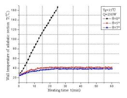
Figure 4. Starting property of inorganic heat transfer element with small inclination angle.
