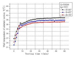
Figure 5. Starting property of inorganic heat transfer element with big inclination angle.
