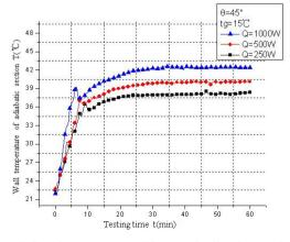
Figure 6. Starting property with same inclination angle and different heating power.
