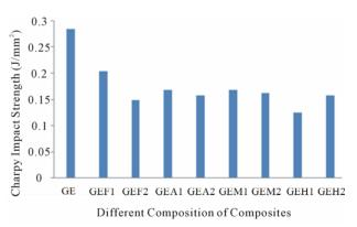
Figure 2. Charpy impact strength for different composition of composite materials.
