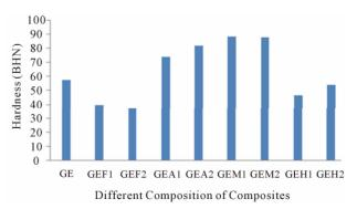
Figure 3. Brinell hardness number for different composition of composite material.
