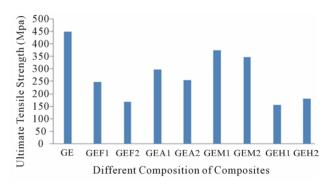
Figure 1. Ultimate tensile strength for different composition of composite materials.
