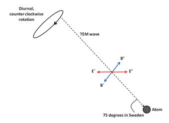
Figure 1. The atom absorbed TEM waves originating from a source towards north and aligned approximately along the earth's rotational axis. The TEM waves were polarized and the electric field vectors were always oriented in the horizontal plane.
