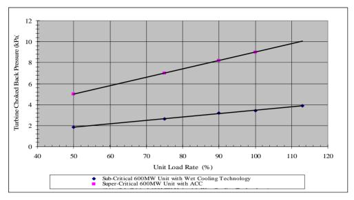
Figure 3. Performance curves of the turbine choked back pressure with unit load.
