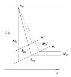
Figure 1. LP turbine expansion line under different LP turbine back pressure operation conditions. condensing steam turbine with ACCs. There are totally
