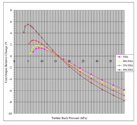
Figure 2. Performance curves of the unit output with turbine back pressure.
