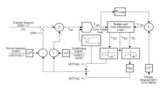
Figure 2. Diagram of DC model CDC6T.
