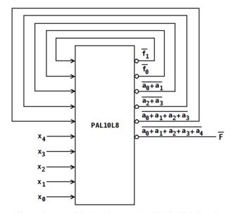
Figure 4. A possible implementation of PAL10L8 circuit.
