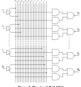
Figure 2. The circuit PAL10L8.
