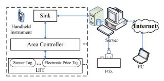
Figure 1. Architecture of Electronic Intelligent Tag System (EITS).
