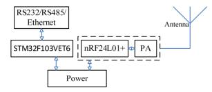
Figure 4. The structure of Sink.
