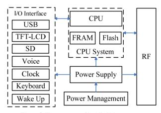
Figure 5. The structure of handheld instrument.
