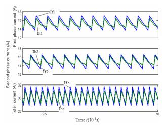
Figure 3. Steady state current waveforms of 2-phase VRM with passivity-based control strategy.
