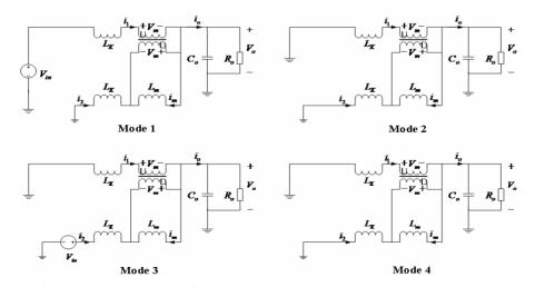
Figure 2. Four operating modes of 2-phase negative coupled planar magnetic integrated VRM.
