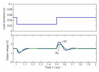
Figure 4. Dynamic response of output voltages of 2-phase VRM with passivity-based control strategy.
