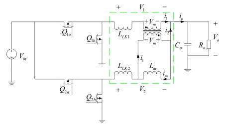
Figure 1. Equivalent circuit of two-phase negative coupled planar magnetic integrated VRM.
