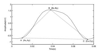
Figure 1. A typical triangle ABC extracted from a signal.
