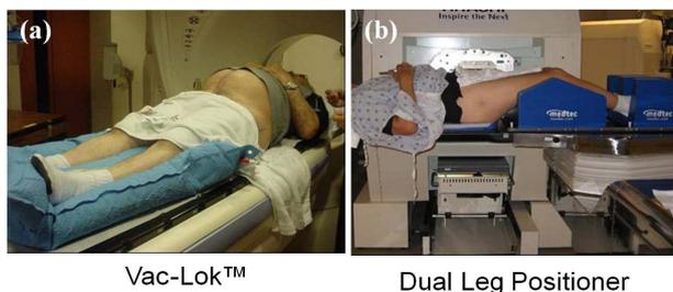
**Figure 1.** Two commercially available pelvic immobilization devices. The Vac-Lok system (a), a patient-specific radiotranslucent cushion that fixes the patient's anatomy from the upper thighs to the feet. The Dual Leg Positioner system (b), a non-patient-specific vinyl-covered foam immobilization device.
